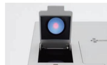
Opening the sample viewer provides a clear, illuminated view of the sample at the measurement port. On the CM-3600A, this view is reflected in a mirror so that you can view it easily even while seated.
