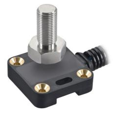
The sensor contains two independent measuring circuits, each with its own power connections, meaning safety critical applications can be addressed. Furthermore, on-board diagnostic functions mean that the outputs can be put into safe, pre-defined states should an internal error be detected.
