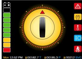
Select the number, size, color and types of instruments. The screen layout and number of instruments will dictate the number and location of warning icons.
