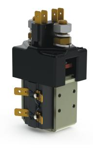
The SW80 has been designed for direct current loads, including motors as used on electric vehicles such as industrial trucks, and telecom and power distribution applications. Developed for both interrupted and uninterrupted loads, the SW80 is suitable for switching Resistive, Capacitive and Inductive loads.
