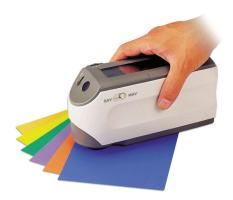
To utilise the DosiXpress<sup>TM</sup> system, the ColorMatrix customer uses a hand held Spectrophotometer, typically a "Konica Minolta CM-2600d", connected to their pc to measure the color values of a sample they wish to match to. The system then evaluates this match against the colorant palette available from ColorMatrix and offers up to 50 formulation options to the customer to choose from.
