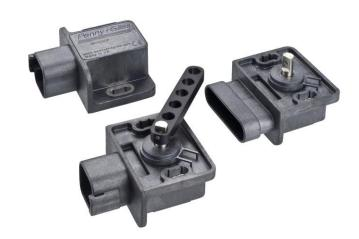
The SRH220DR is a shaft-operated, No Contact rotary position sensor with dual-redundant outputs. The versatile, factory-programmable electronics, which can be supplied from 5V or 9-30V, can be easily set to one of three analog voltage output ranges or one of three PWM frequencies. In addition, the polarities of the analog outputs can be set to one of three combinations – both tracking in the same direction or one opposite to the other.
