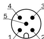
Connector M12, 5-pin, A-coded
