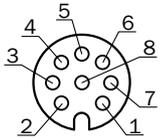
Connector M12, 8-pin, A-coded
