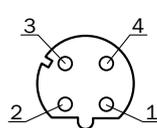
M12 female connector, 4-pin, D-coded
