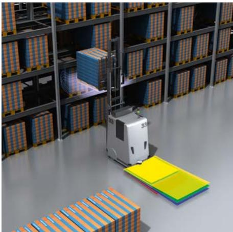
Smooth processes are essential in high-bay warehouses. Free storage spaces must be filled quickly and without complications. The MRS1000 enables exact positioning of transport forks in automated guided vehicle systems (AGVs), making collision-free movement into a free space possible. When moving backwards, the MRS1000 detects objects protruding into the space with its several scanning layers, ensuring reliable collision protection.
