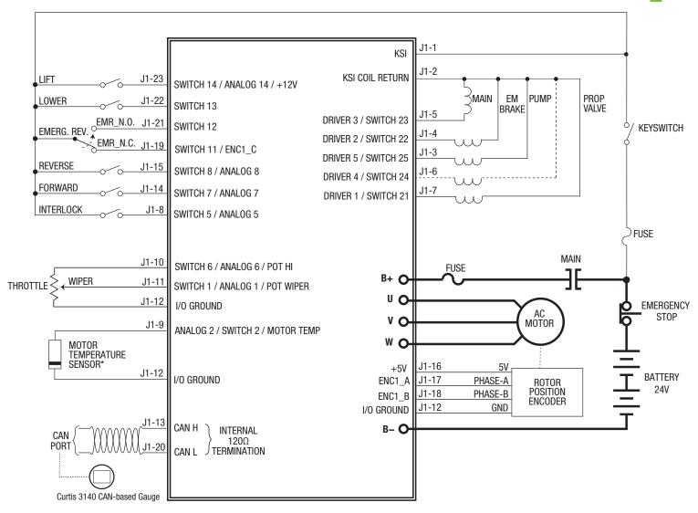
\*NOTE: KTY sensor shown. The banded end must be connected to I/O Ground.
